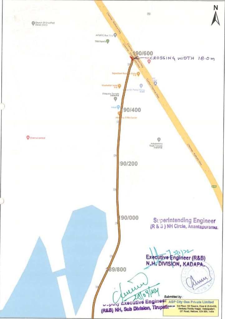
Map Showing Details of Proposed Pipeline Along NH-71 from Ch:190/600 to 187/360
